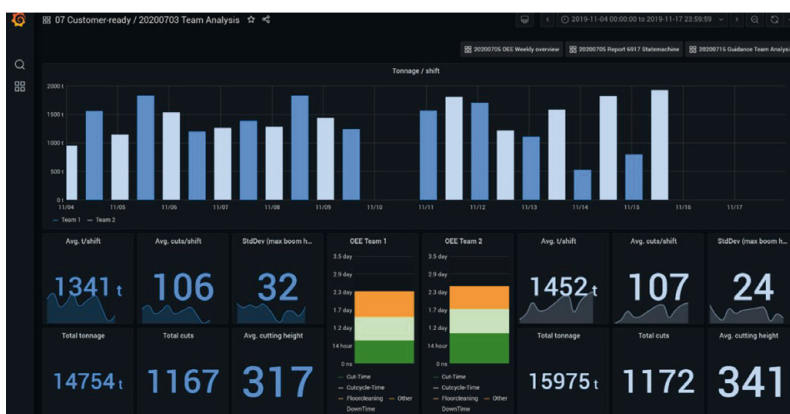
Fig. 11: Analysis of the quantities of coal produced by different groups of continuous miner operators
